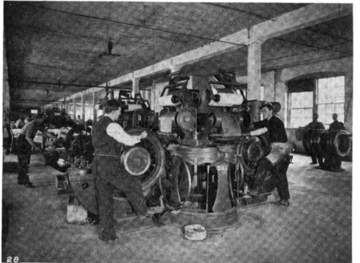
A View of the Goodyear Tire-Making Machine, Showing Operators on Each Side Stretching Fabric.
